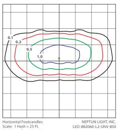
Scale: 1 Hash = 25 Ft. Light Loss Factor = 1.00 Total Lamp Lumens = 6139.63 Mounting Height = 25.00 Ft., Tilt = 5 Degrees Maximum Calculated Value = 1.43 Fc Arrangement: Single
